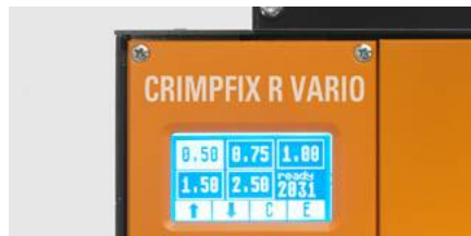
One-touch adjustment between cross-sections
