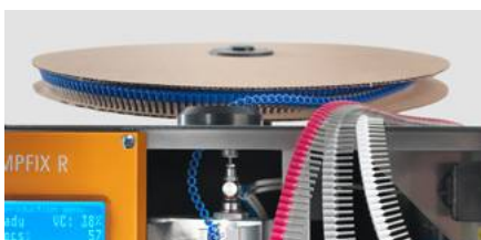
Automatic cross-section adjustment from 0.5 to 2.5 mm 2
