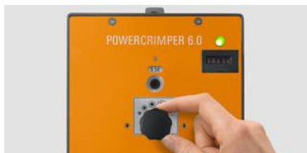
Tool-less change to different wire-end ferrule types
