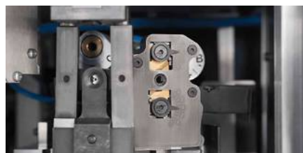
Adjustable stripping blade for the best stripping quality
