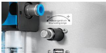
Individual adjustment of the cable holding force
