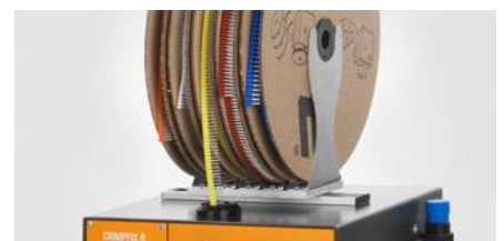
Processing of linked, reeled wire-end ferrules
