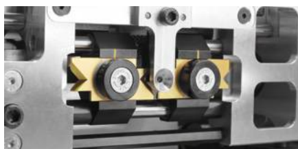
Stripping blade can be used on both sides
