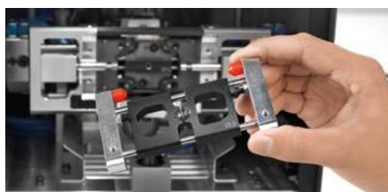
Quick-change tool for extremely short retooling times
