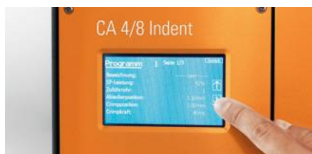
Automatic adjustment of the stripping length and crimp depth
