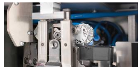
Adjustable trigger sensor for optimum stripping length
