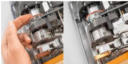
Simple mechanical changeover for cross-section change
