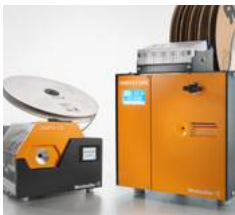
8 Automatic strippers and crimpers for wire-end ferrules on reel
