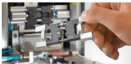
Quick-change tool for extremely short retooling times
