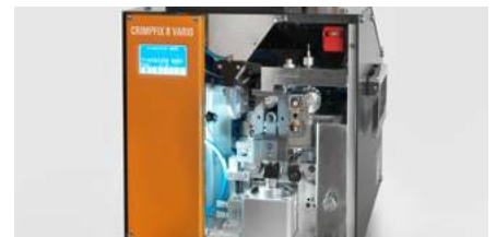
Adjustment to various crimping lengths (8 mm and 10 mm)
