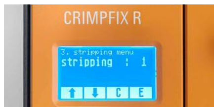
Separate stripping mode adjustable
