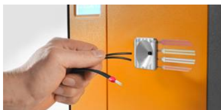
Stripping and crimping in one step
